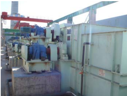
热轧油环废水处理稀土磁盘 Rare earth magnetic disc for contact water treatment system for hot rolling mill
