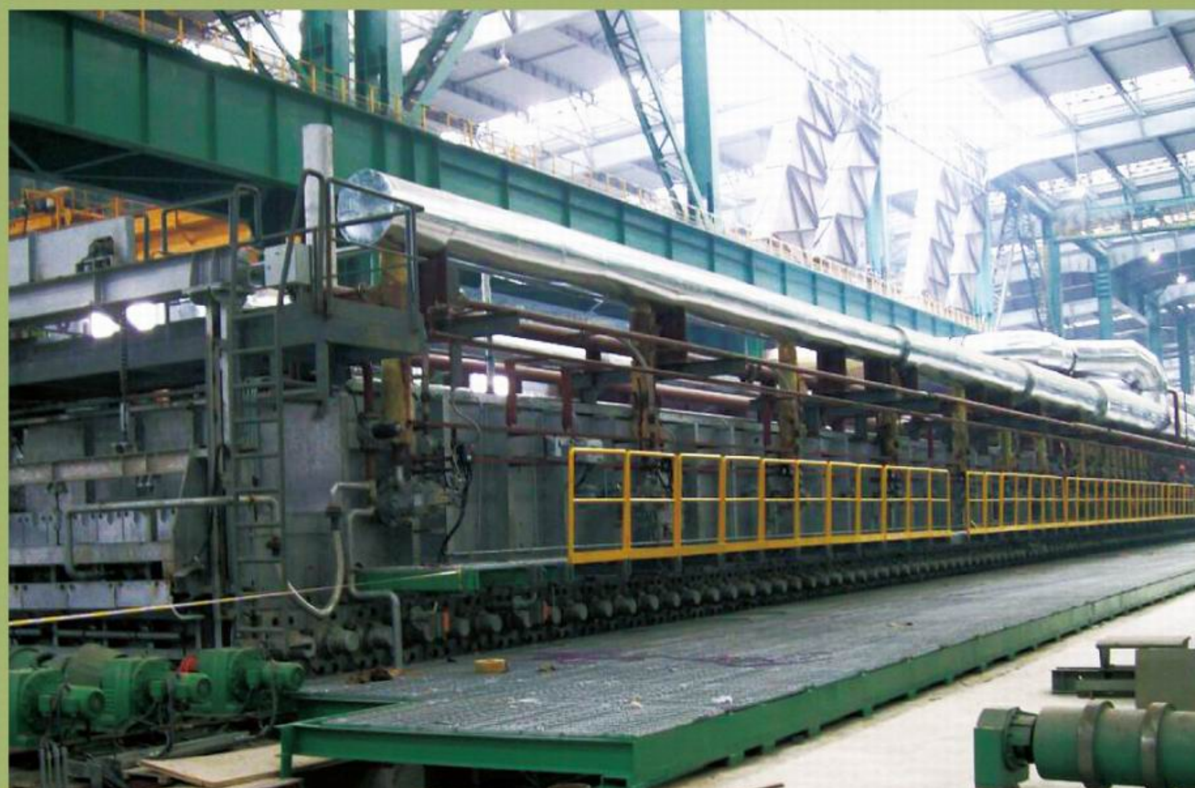
首钢中厚板辊底式热处理炉（保护气体） Roller hearth heat treatment furnace for medium and thick plate mill Shougang (protective gas)
